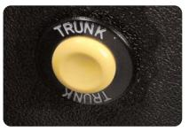
To unlock your trunk, press the button located behind the glove box door. You can also unlock the trunk by pressing the car symbol shown on your Remote Keyless Entry transmitter. Or, simply use your door key to open the trunk.
