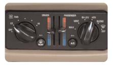
The left knob operates the fan and provides five speed settings ranging from LO to HI. The knob on the right offers six operating modes:
