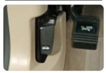
Pull the hood release handle located under the driver's side of the instrument panel.
