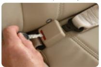
Pull forward on the seatback tab on the outboard of the rear seat cushion and fold the seatback down.
