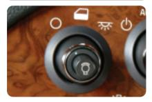
The interior lamps control is located next to the exterior lamps control on the left side of the instrument panel. It can be set to:
