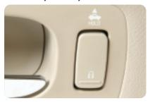
To unlock the trunk from inside the vehicle, press and hold the top of the driver's or front passenger's power door lock switch for approximately two seconds. The vehicle must be in Park to unlock the trunk.
