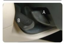
To adjust the tilt position of the steering wheel, hold the wheel and pull the lever (see "A") on the left of the steering column toward you. Move the wheel up or down to a comfortable level. Release the lever to lock.
