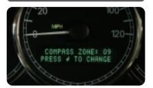
The base-level Driver Information Center (DIC) displays the odometer and trip odometer. Uplevel DICs also display a compass, trip computer, fuel economy information, OnStar® phone numbers called (if equipped) and other messages or warnings. The DIC display is located on the instrument cluster below the speedometer, and can be programmed in English, French or Spanish.
