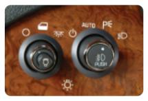
You will find the exterior lamps knob on the left side of the instrument panel.
