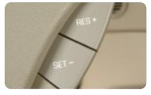
The cruise control buttons are located on the steering wheel.
