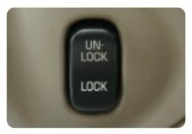
Press UNLOCK or LOCK on the door switch to unlock or lock all of the doors.
