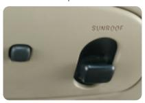
The sunroof switch is located on the headliner, between the sun visors.
