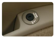
Press the TRUNK RELEASE button to open the trunk lid.
