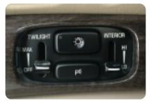
The Twilight Sentinel control lever is located to the left of the steering column. To operate it, slide the lever from OFF to MAX to adjust the headlamps ON time from a few seconds to three minutes, after the ignition has been turned OFF.
