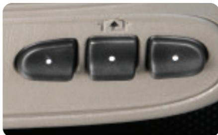
This programmable transmitter can store up to three frequencies for items such as a garage door opener, entry door lock or security system. With the ignition OFF, program the transmitter as follows:
