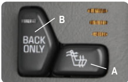
**Heated Seats (if equipped):** The buttons to control this feature are located on the front door armrests. Controls can be set to heat the seatback only or the seatback and the seat cushion. The three lights next to the controls indicate LO, MED or HI setting. Push the BACK ONLY switch ("B" above) to activate heat for the seatback only. An indicator light illuminates when the seatback is being heated. Push the horizontal switch ("A" above) to heat the whole seat.
