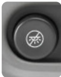
Although using your Remote Keyless Entry transmitter to unlock the doors will activate the dome lamp temporarily, the lamp will remain deactivated when opening a door, until the override button is pressed again.
