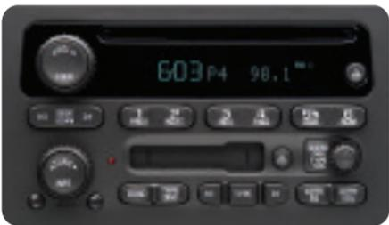
**Setting the Clock:** Press and hold the H (or HR) button until the correct hour appears. AM or PM will appear on the radio display. Press and hold MN until the correct minute appears.
