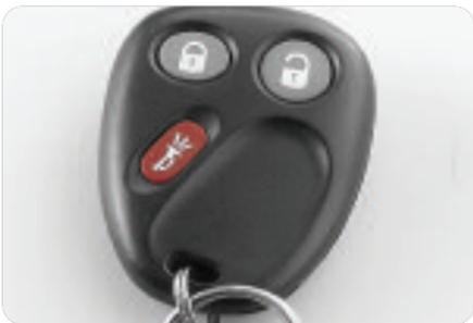
The RKE system locks and unlocks the doors and lift glass from a range of 3 to 30 feet (1–9 m). At times the range may be shorter than usual, which is normal. If the transmitter doesn't seem to be working properly:
