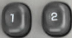
Use the driver's door mounted controls (shown above) to program and recall memory settings for the following features:
