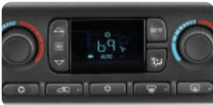
Your vehicle is equipped with a climate control system that automatically maintains the desired temperature individually for the driver and front seat passenger. Independent rear seat fan and air distribution controls are also included for increased rear-passenger comfort. A memory feature for up to two drivers is also included with this system.
