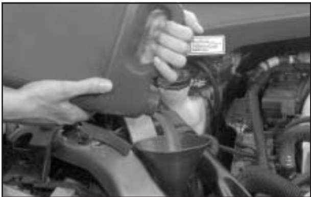
Filling in the Radiator Filler Neck
