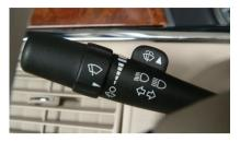
The windshield wipers/washer controls are located on the multifunction lever on the left side of the steering wheel.
