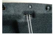
Use the deck lid tie-down to secure the deck lid when carrying oversize cargo that prevents the deck lid from closing completely. Observe all applicable safety precautions.
