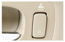
To unlock the trunk from inside the vehicle, press and hold the top of the driver's or
