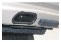
A convenient handle is located in the top-inside edge of the deck lid. Use the handle to easily pull down the deck lid when closing it.
