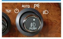
You will find the exterior lamps knob on the left side of the instrument panel.
