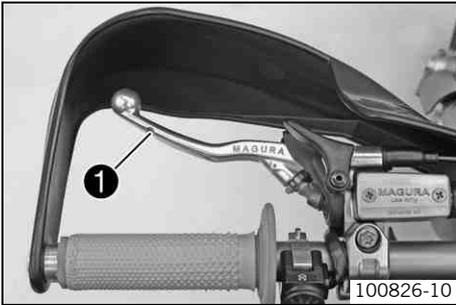
The clutch lever ❶ is fitted on the left side of the handlebar. The clutch is hydraulically operated and self-adjusting.
