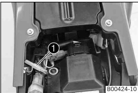
The plug connection ❶ is located under the seat near the upper shock absorber fixation.
