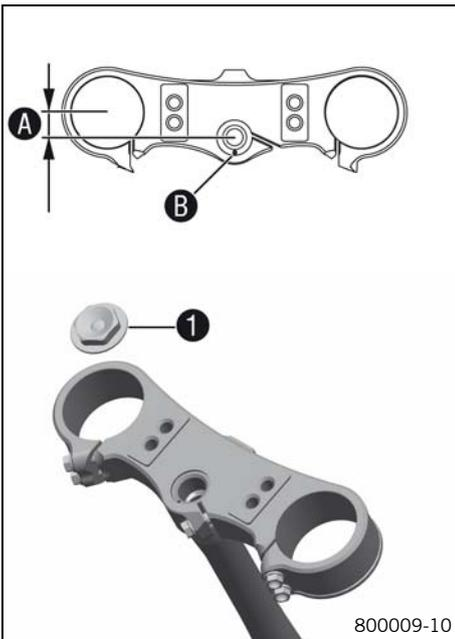
You can see the currently set offset if you remove screw ❶. The fork offset A has an impact on the handling of the vehicle. It is calculated from the center of the fork leg to the center of the steering head bearing. The fork offset can optionally be adjusted. Marking B to the front gives greater stability on fast racetracks.
