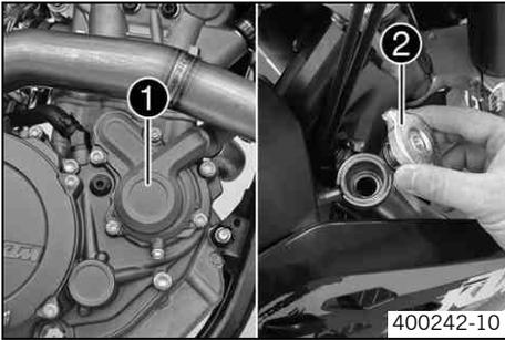
Water pump ❶ in the engine circulates the coolant.
