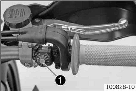
Electric starter button ❶ is fitted on the right side of the handlebar.
