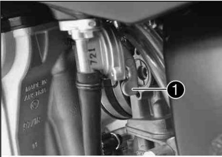
With the tap handle ❶ on the fuel tap, you can open or close the supply of fuel to the carburetor.
