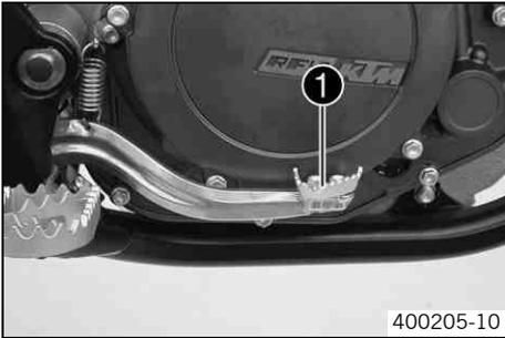
Foot brake lever ❶ is located in front of the right footrest. The foot brake lever is used to activate the rear brake.
