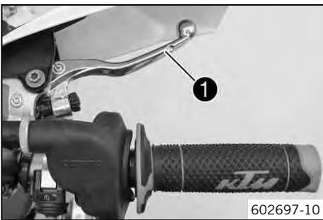
Hand brake lever ❶ is located on the right side of the handlebar. The hand brake lever is used to activate the front brake.
