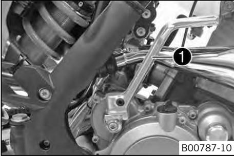
The kick starter ❶ is fitted on the right side of the engine. The top part can be swiveled.
