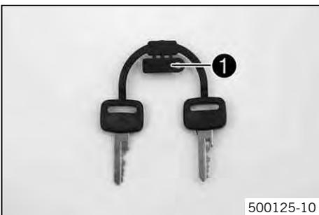
The key number ❶ for the steering lock is stamped onto the key connector.
