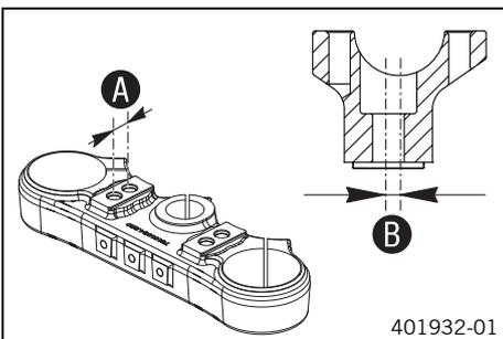
On the upper triple clamp, there are two holes a distance of **A** apart.
