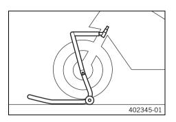
Move the handlebar to the straight-ahead position. Position the lifting gear.
