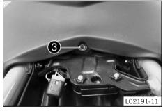
Mount and tighten screw 3 with the washer.
