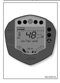
If the fuel level drops to the reserve mark, the display mode automatically changes to **TRIP F** and starts to count from **0.0**, regardless of the previous display mode.
