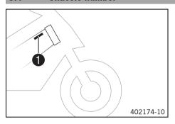
The vehicle chassis number **1** is stamped on the frame behind the steering head on the right.
