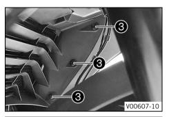
Remove expanding rivet 3.
