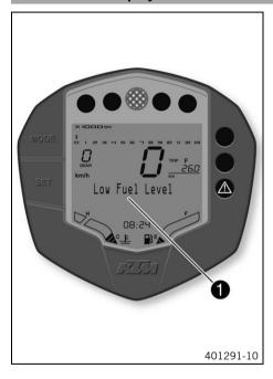
Various warning notes appear on info display ①. If the general warning lamp ⓐ lights up, the corresponding warning note is shown on the info display.
