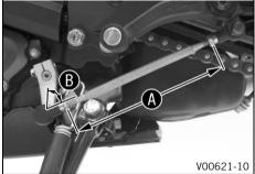
Loosen nut 1, holding threaded rod 2.
