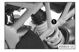
Set the spring pretension by turning adjusting ring 1 using the hook wrench and the extension from the tool set.
