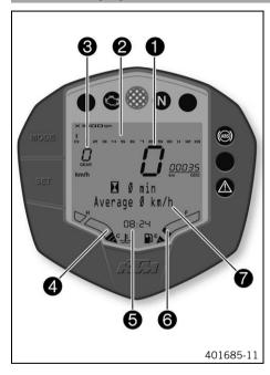
The speed 1 is shown in kilometers per hour **km/h** or in miles per hour **mph**.
