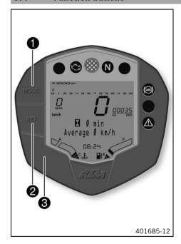
You can change the display mode with the **MODE** button **1**. Possible display modes are total distance traveled (**TRIP 1**), distance 1 (**0D0**) and distance 2 (**TRIP 2**).
