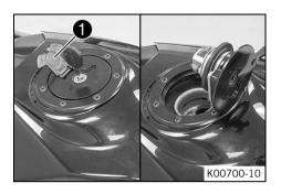
Lift the cover 1 of the filler cap and insert the ignition key in the lock.
