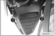
Mount and tighten screws 2.
