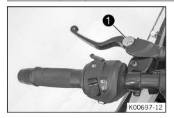
Adjust the basic position of the clutch lever to your hand size by turning adjusting wheel
