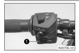
The horn button 1 is fitted on the left side of the handlebar.
