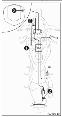
The ABS unit ①, which consists of a hydraulic unit, ABS control unit, and return pump, is installed under the seat. One wheel speed sensor ② is located in each case on the front and the rear wheel
