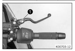
Adjust the basic position of the hand brake lever to your hand size by turning adjusting wheel 1.
