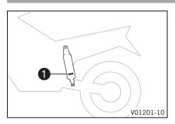
Shock absorber article number **1** is on the left side of the shock absorber.
