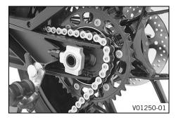
Push the rear wheel forward as far as possible. Remove the chain from the rear sprocket.
