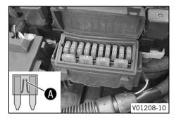
Remove the faulty fuse.
