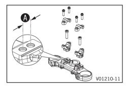
On the upper triple clamp there are two holes at a distance of **A** apart.
