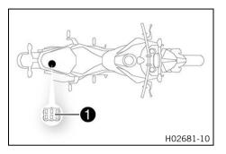
Diagnostics connector **1** is located under the passenger seat.
