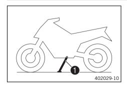
The side stand **1** is located on the left of the vehicle. The side stand is used for parking the motorcycle.
