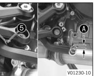
Loosen nut 4 and turn screw 5 correspondingly until the free travel A is present. If necessary, adjust the basic position of the foot brake lever.
