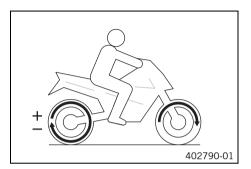
The slip adjustment is a motorcycle traction control function. The slip adjustment allows the motorcycle traction control to be tuned through nine levels to the desired characteristic map. Level 1 allows the maximum slip on the rear wheel, and level 9 the minimum
