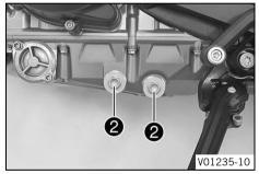
Remove oil drain plugs with the magnets, O-rings, and oil screens.
