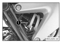
Set the spring preload by turning at the adjusting device using the hook wrench from the tool set.
