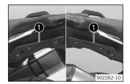
The case holders **1** are located on each side of the passenger seat.
