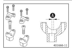
The holes on the handlebar support are placed at a distance of **A** from the center.
