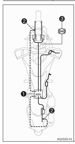
The ABS unit ①, which consists of a hydraulic unit, brake electronics control unit, and return pump, is installed under the seat. One wheel speed sensor ② is located in each case on the front and the rear wheel.
