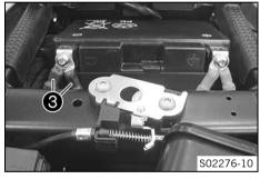
Disconnect both negative cables 3 of the battery to avoid damage to the motorcycle's electronics.
