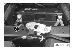
Connect both negative cables **3** to the battery. Guideline
