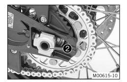
Push the wheel spindle in all the way and mount chain adjuster 4 and nut 5.
