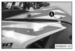
Position the side cover in the area under the tank cover.
