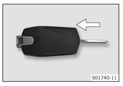
Fit lower half of the Race-on key and snap into place in the direction of the arrow.
