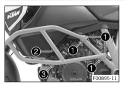
Position the left crash bar with frame protector and attach the clamp to the frame tube.
