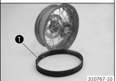
This vehicle makes use of a tubeless tire system in which a tubeless sealing profile **1** is used instead of the conventional tube. The advantage of the tubeless system is that there is no risk of a defective tube. This greatly reduces the risk of a sudden loss in pressure.
