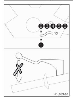
If the  $\underline{\text{quickshifter +}}$  (optional) is activated, you can shift up and down without actuating the clutch.
