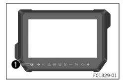
The Race-on indicator lamp ① can indicate errors by flashing. The flashing occurs for up to five seconds after actuating the Race-on tip switch.
