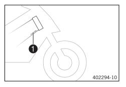
The chassis number **1** is stamped on the bottom right of the frame behind the steering head.
