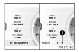
The ice symbol  $\circledast$  is shown in area 1 of the display. The ice symbol  $\circledast$  appears on the display when the ambient temperature drops below the specified value.
