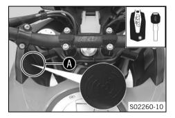
On this vehicle, the ignition/steering lock is replaced by a remote key with transponder (Race-on key (19 p. 51)).
