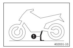
In addition to the side stand, the vehicle is equipped with a center stand  $\ensuremath{\text{1}}$ .
