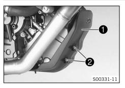
Position engine guard 1, mount screws 2 with bushings and tighten.
