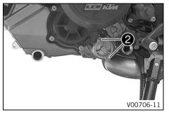
Mount and tighten screws 2.
