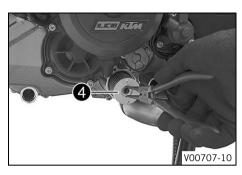
Pull oil filter 4 out of the oil filter housing.
