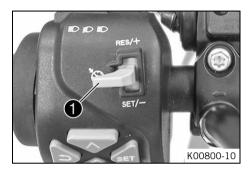
The cruise control system tip switch **1** is fitted on the left side of the combination switch.
