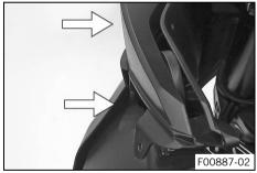
Position the mask spoiler and press laterally into the supports.
