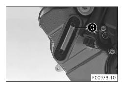
Remove the screw plug and add the second partial quantity up to the upper marking on the engine oil level viewer.
