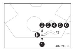
The gear positions can be seen in the figure.
