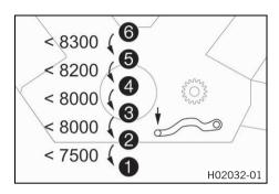
If the quickshifter + is enabled in the combination instrument, you can shift down in the speed range shown without pulling the clutch lever.
