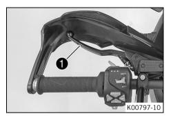
The clutch lever **1** is fitted on the left side of the handlebar. The clutch is hydraulically operated and self-adjusting.
