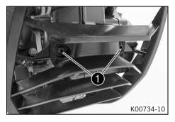
Position the front spoiler. Mount screws but do not tighten yet.
