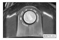
The ignition/steering lock is in front of the upper triple clamp.
