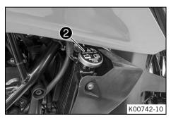
Remove radiator cap 2 and check the coolant level in the radiator.
