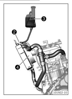
The coolant is cooled by the air stream and a radiator fan  $oldsymbol{4}$ , which is activated at high temperature.
