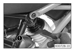
Adjust the spring preload by turning adjusting ring ①.
