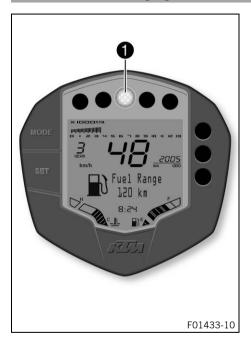
The shift warning light **1** is located in the center above the display.
