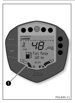
The coolant temperature display is shown in segment **1** of the display.
