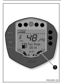
The fuel tank contents are shown in area **1** of the display. The fuel level indicator consists of bars. The more bars are lit, the more fuel is in the fuel tank.
