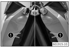
Mount expanding rivets 1 on both sides.
