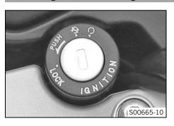
The ignition and steering lock is located in front of the upper triple clamp.
