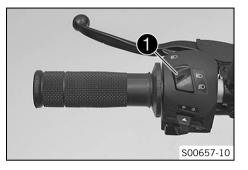
The light switch 1 is fitted on the left side of the handlebar.
