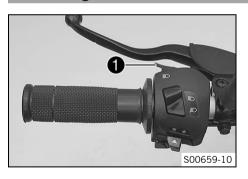
High beam flasher button **1** is fitted on the left side of the handlebar.
