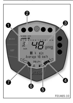
The tachometer **1** shows the engine speed in revolutions per minute.
