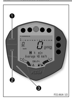
Press the **MODE** button **1** to change display modes. Possible display modes are **TRIP F** (after reaching the fuel reserve level), total distance traveled **(0D0)**, distance 1 **(TRIP 1)** and distance 2 **(TRIP 2)**.
