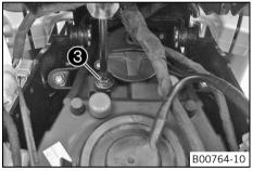
Adjust the beam headlight range by turning screw 3.
