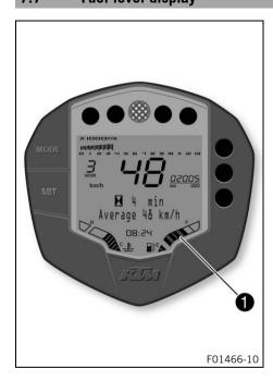
The fuel tank contents are shown in area **1** of the display. The fuel level indicator consists of bars. The more bars are lit, the more fuel is in the fuel tank.
