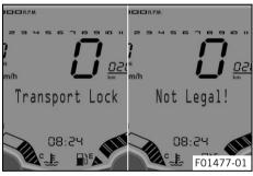
**Transport Lock** appears on the display if transport mode is activated.
