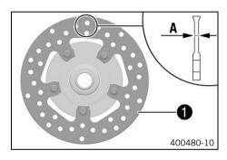
Check the front and rear brake disc thickness at multiple points for the dimension A.
