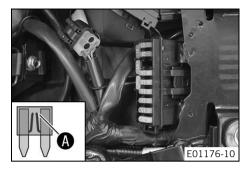
Remove the faulty fuse.
