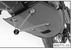
Mount and tighten screws 2.
