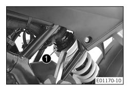
Set the spring pretension by turning adjusting ring using the hook wrench from the tool set.
