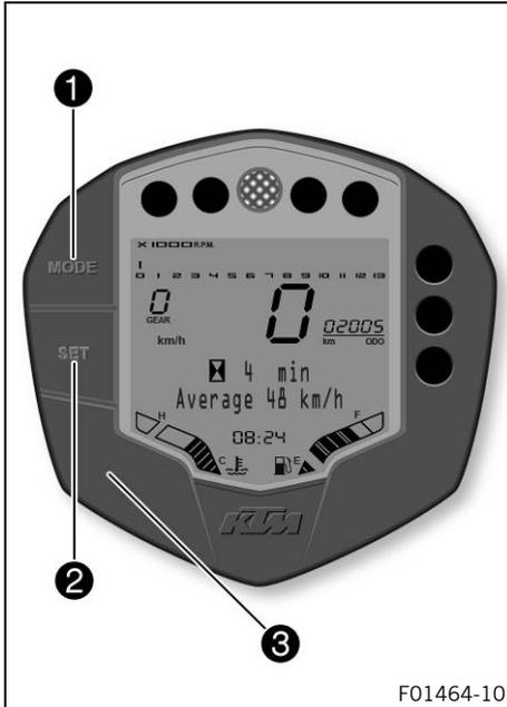
Press the **MODE** button **1** to change display modes. Possible display modes are **TRIP F** (after reaching the fuel reserve level), total distance traveled (**ODO**), distance 1 (**TRIP 1**) and distance 2 (**TRIP 2**).
