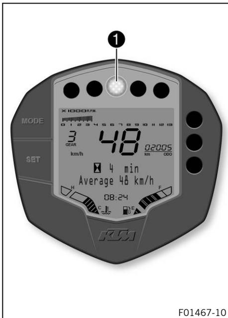
The shift warning light ① is located in the center above the display.
