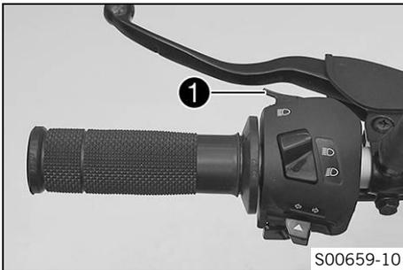
High beam flasher button ① is fitted on the left side of the handlebar.
