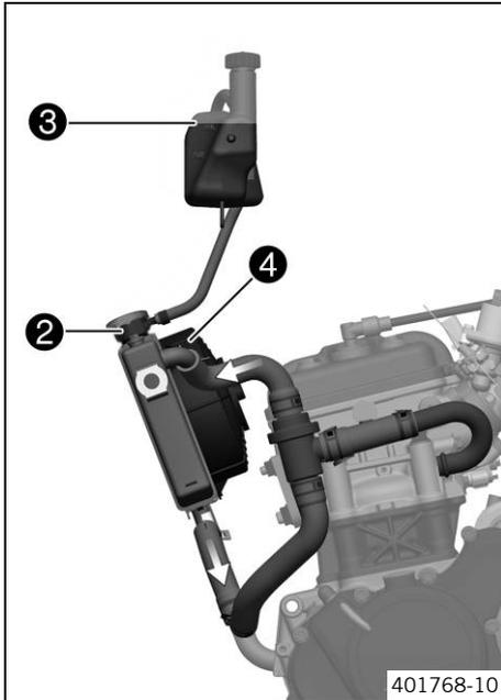
The coolant is cooled by the air stream and a radiator fan ④, which is activated at high temperature. The lower the speed, the less the cooling effect. Dirty cooling fins also reduce the cooling effect.
