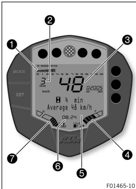
The tachometer ① shows the engine speed in revolutions per minute.
