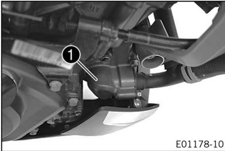
Water pump ❶ in the engine ensures forced circulation of the coolant.
