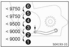
If the <u>quickshifter +</u> (optional) is enabled in the combination instrument, you can shift up in the speed range shown without pulling the clutch lever.
