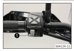
Horn button **1** is fitted on the left side of the handlebar.
