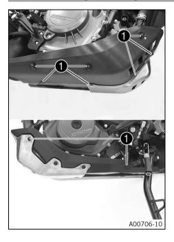
Position the engine guard, mount and tighten screws 1.
