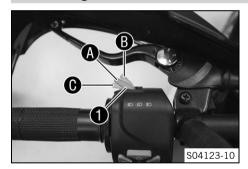
Light switch 1 is fitted on the left side of the handlebar.
