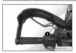
Adjust the basic position of the clutch lever to your hand size by turning adjusting wheel 1.
