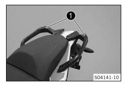
The grab handles **①** are used for moving the motorcycle around. If you carry a passenger, the passenger can hold onto the grab handles during the trip.
