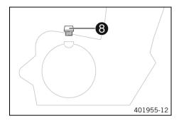
Remove filler plug **8** with the O-ring, and fill up with engine oil.
