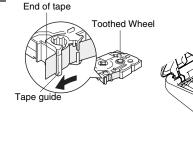
Make sure that the end of the tape feeds under the tape guides. • If the ink ribbon is loose, use your finger to wind the toothed wheel in the direction of the arrow on the cassette
