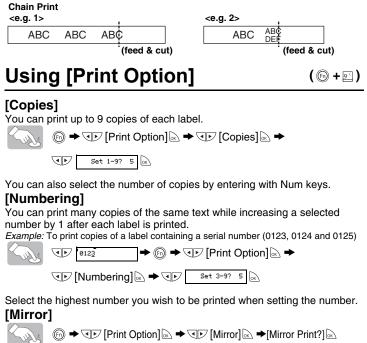
J.SMITH Use a clear tape in [Mirror], so the labels can be read correctly from the opposite side when attached on glass, windows or other transparent surfaces.
