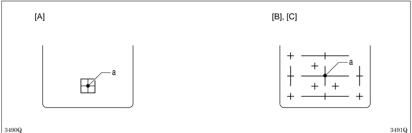
5. Turn the pulley by hand and check at what point the needle drops to the home position standard plate. If the needle does not drop to point (a), carry out the following adjustments.
