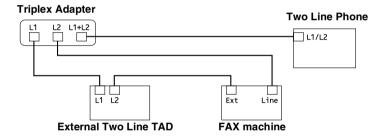
You can keep two-line telephones on other wall outlets as always. There are two ways to add a two-line telephone to the fax machine's wall outlet. You can plug the telephone line cord from the two-line telephone into the L1+L2 jack of the triplex adapter. Or, you can plug the two-line telephone into the TEL jack of the two-line TAD.
