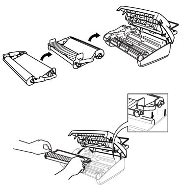
Press down on both sides of the top cover to close it securely.
