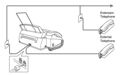
Whenever this external phone (or TAD) is in use, the screen displays  ${\tt EXT}$ .  ${\tt TEL}$   ${\tt IN}$   ${\tt USE}$ , and, if the fax handset is lifted, an alarm sounds.
