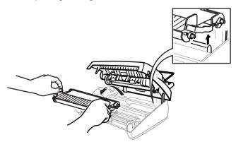
4 To clean your machine's print head, wipe the print head with a lint-free cloth that is dry or lightly moistened with isopropyl alcohol.
