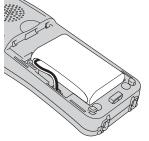
3 Install the battery cover by sliding it onto
