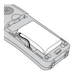
5 Install the battery cover by sliding it onto the back of the handset.
