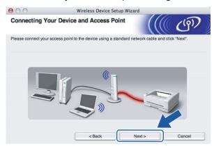
9 Choose the printer you wish to configure, and click Next. If the list is blank, check if the access point and the printer are powered on, and then click Refresh.
