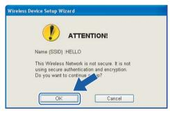
14 If your network is configured for Authentication and Encryption, the following screen will appear. When configuring your Brother wireless printer, you must ensure that it is configured to match the Authentication and Encryption settings of your existing wireless network. Choose the Authentication Method and Encryption Mode from the pull-downs in each setting box. Then enter the Network key and Confirm Network Key, and then click Next.
