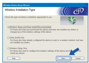
Wireless configuration for Windows® using the Brother installer application (For HL-2170W)
