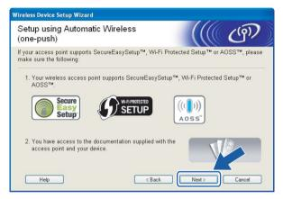
Press the wireless setup button located at the back of the machine for less than 2 seconds as show in the illustration below. This will put the printer in one-push wireless setting mode. This feature will automatically detect which mode your access point uses for one-push configuration (SecureEasySetup™, Wi-Fi Protected Setup™ or AOSS™) of your printer.
