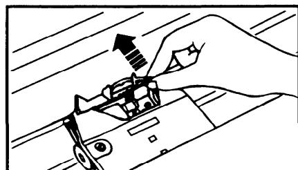
**Note:** Please check the shape of your daisy wheel cassette before replacing the daisy wheel. The daisy wheel cassette type B cannot be used with this machine.
