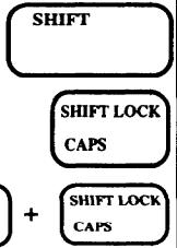
For continuous uppercase typing: Press [SHIFT LOCK] (the SHIFT lamp will blink and all the keys will be set in uppercase mode). To return to lowercase typing, press either the right or left [SHIFT] key.
