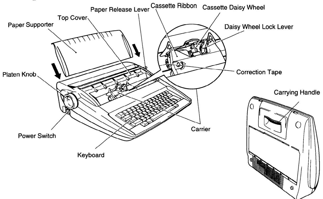
**Paper Release Lever:** Pushing this lever loosens tension on the paper so it can be adjusted if necessary.
