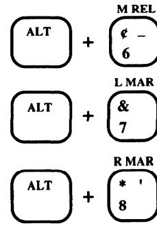
To move beyond the position of a current margin, first position the carrier on the margin and press [ALT] + [M REL].
