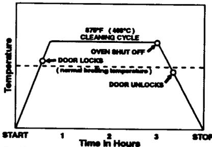
The Self-Cleaning cycle uses very high heat to burn away soil and grease. During the cycle, the oven gets much hotter than it does for normal baking or broiling. This high heat breaks up the soil or grease and burns it away.
