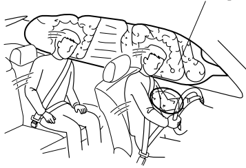
The side air bag will deploy only on the side the vehicle receives the force of the impact.
