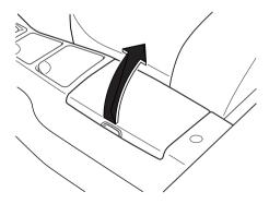
To release the trunk lid, pull up on the trunk lid release lever.
