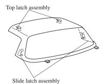
5. Align the rear deck latches with the rear deck studs and set the hardtop squarely onto the body.
