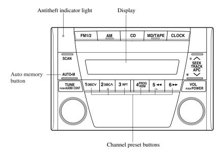
To deter theft of your vehicle's audio unit, it has an integrated antitheft system. The system is designed to accept a code number that makes the unit inoperable if it is stolen.
