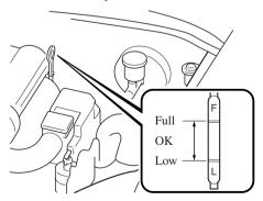
Pull it out again and examine the level. It's OK between L and F. But if it's near or below L, add enough oil to bring the level to F.
