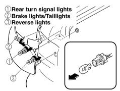
4. Install the new bulb in the reverse order of removal.
