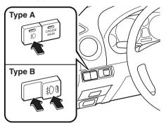
To turn on the fog lights, first turn the headlight switch to the ♣○♣○ position. Then press the fog light switch. To turn the fog lights off:
