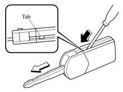
2. Insert a small screwdriver into the slot and gently pry open the transmitter.
