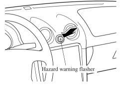
Depress the hazard warning flasher and all four turn signals will flash.
