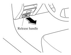
2. Pull the hood latch up and lift the hood.
