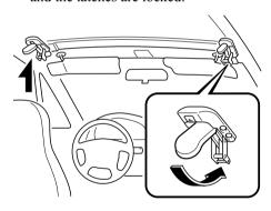
8. Push each side latch down with the palm of your hand until the lock buttons click and the latches are locked.
