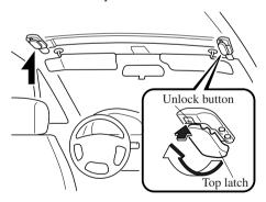
5. Push the unlock buttons and fully release the side latches.
