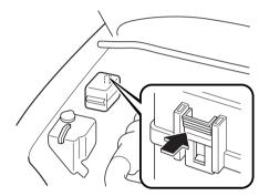
3. If a fuse is blown, replace it with a new one of the same amperage rating.
