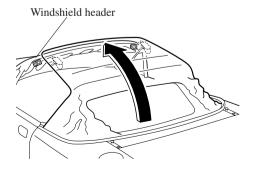
8. After securely hooking the top latches onto the windshield header, push each latch up with the palm of your hand until the lock buttons click and the latches are locked
