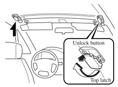
6. Lift up on the front section of the top to release it from the windshield header.
