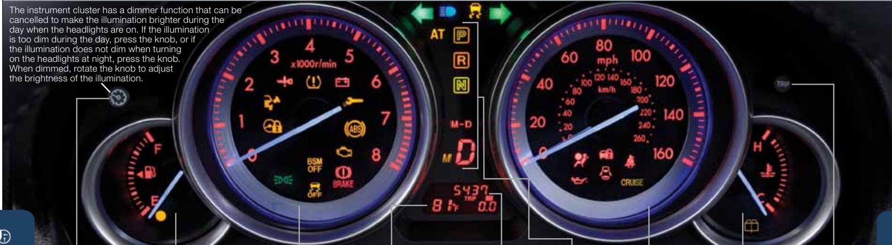
INSTRUMENT CLUSTER DIMMER 1 FUEL GAUGE TACHOMETER AMBIENT TEMPERATURE 2 ODOMETER/ TRIP METER SHIFT LEVER POSITION INDICATOR SPEEDOMETER ENGINE COOLANT TEMPERATURE GAUGE TRIP METER SELECTOR 2,3
