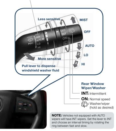
**CAUTION:** When the ignition is ON, turn the AUTO wipers OFF when going through a car wash, or while cleaning or touching the windshield.
