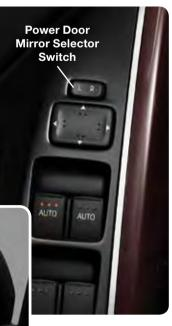
**NOTE:** If the left/right power outside mirror selector switch is in the center position, or the selector lever is shifted to a position other than the R position, the outside mirrors return to their on-road position automatically. The door mirrors return to their on-road position automatically even when the ignition is switched from ON to OFF.
