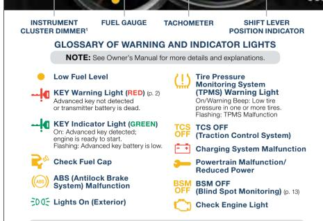
**TPMS NOTE:** Low ambient temperature and/or high altitude causes tire pressures to drop and may turn the TPMS warning light on. If the warning light comes on, check the tire pressure and fill the tires as soon as possible, preferably before moving the vehicle and warming up the tires. Tire pressure should be checked when the tires are cold.
