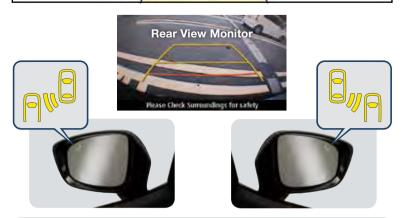
**WARNING:** RCTA is only a supplementary system to help aid when backing up, however RCTA has limitations. The system does not detect all vehicles. Do not rely solely on the RCTA. Relying solely on the RCTA may cause an unexpected accident resulting in serious injury. Always back up slowly.
