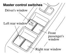
To open the window to the desired position, hold down the switch. To close the window to the desired position, pull up the switch.
