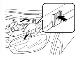
3. If any fuse but the MAIN fuse is blown, replace it with a new one of the same amperage rating.
