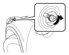
5. Install the new bulb in the reverse order of the removal procedure.
