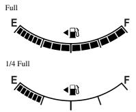
If the low fuel warning light illuminates or the fuel level is very low, refuel as soon as possible.
