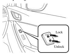
To lock all the doors/liftgate from an open front door, press the lock side of the door lock switch and then close the door.
