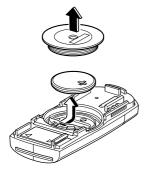
5. Insert a new battery with the positive pole facing up, and then cover the battery with the battery cap.
