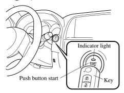
4. After the push button start indicator light (green) changes to full illumination, press the push button start with your finger.
