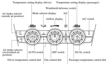
Mode selector switch Rear window defogger switch
