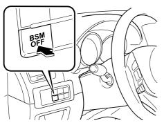
Press the BSM OFF switch again to turn on the BSM system. The BSM OFF indicator light turns off.
