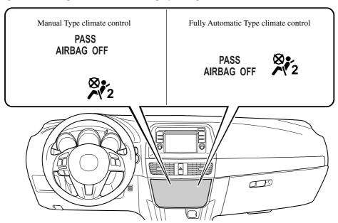
If the front passenger weight sensors are normal, the indicator light illuminates when the ignition is switched ON. The light turns off after a few seconds. Then, the indicator light illuminates or is off under the following conditions:
