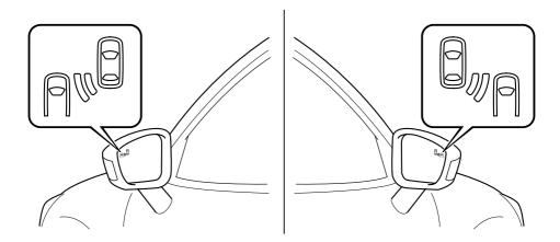
This warning light illuminates for a few seconds when the ignition is switched ON. If the BSM system detects a vehicle in the detection area while the vehicle is driven at a speed of about 32 km/h (20 mph) or more, the BSM warning light illuminates on the side of the vehicle where the rear on-coming vehicle is detected.
