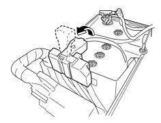
2. Make sure the booster battery is 12 V and that its negative terminal is grounded.
