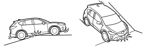
Your vehicle is equipped with low profile tires allowing class-leading performance and handling. As a result, the sidewall of the tires are very thin and the tires and wheels can be damaged if driven through potholes or on rough/uneven roads at excessive speeds. Use care and reduce speed when traveling on rough/uneven roads or through potholes.
