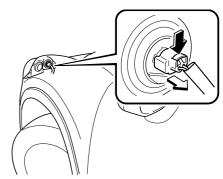
Turn the socket and bulb assembly to remove it. Carefully remove the bulb from its socket in the reflector by gently pulling it straight back out of the socket.
