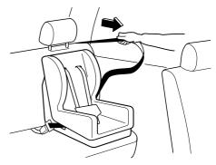
5. Push the child-restraint system firmly into the vehicle seat. Be sure the belt retracts as snugly as possible. A clicking noise from the retractor will be heard during retraction if the system is in the automatic locking mode. If the belt does not lock the seat down tight, repeat this step.
