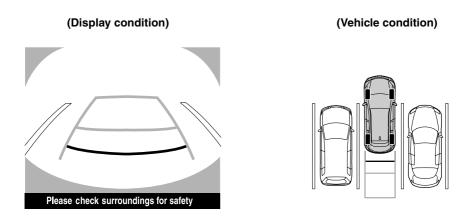
6. When the shift lever is shifted from R to another shift lever position, the screen returns to the previous display.
