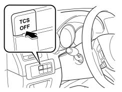
Press the switch again to turn the TCS back on. The TCS OFF indicator light will turn off.
