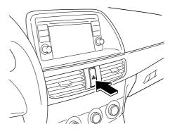
Depress the hazard warning flasher and all the turn signals will flash. The hazard warning indicator lights in the instrument cluster flash simultaneously.
