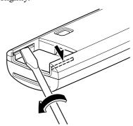
3. Insert the small, flathead screwdriver into the gap between the cover and the transmitter, and then rotate the screwdriver to detach the cover.
