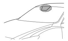
Always keep the surface of the windshield around the laser sensor clean to assure proper operation of the Smart City Brake Support (SCBS) system.
