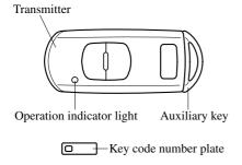
Pull out the auxiliary key from the key (transmitter).
