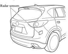
Always keep the bumper surface near the radar sensor area clean so that the BSM system operates normally. Refer to Exterior Care on page 6-56.
