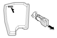
4. Inspect the fuse and replace it if it is blown.
