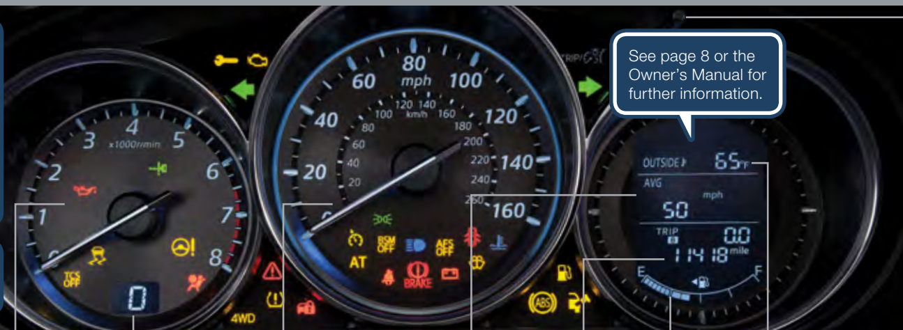
TACHOMETER SHIFT POSITION INDICATOR LIGHT SPEEDOMETER INFORMATION DISPLAY ODOMETER/TRIP METER FUEL GAUGE AMBIENT TEMPERATURE DASHBOARD ILLUMINATION/DIMMER/TRIP METER 2
