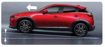
When the brake pedal is released and the accelerator pedal is pushed, HLA prevents the vehicle from rolling forward or backward. It operates on a downward slope when the shift lever is in the reverse (R) position, and on an upward slope when the shift lever is in a position other than the reverse (R) position.
