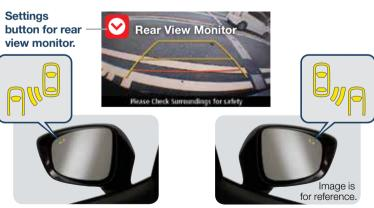
**WARNING:** RCTA is only a supplementary system to help aid when backing up; however, RCTA has limitations. The system does not detect all vehicles, especially a motorcycle. Do not rely solely on the RCTA. Relying solely on the RCTA may cause an unexpected accident resulting in serious injury. Always back up slowly.
