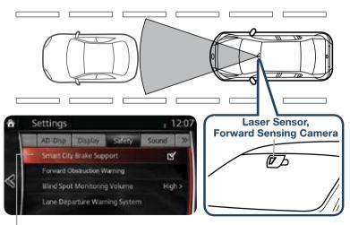
SCBS system can be turned off using Safety Settings in MAZDA CONNECT. (p. 8)
