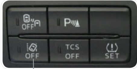
Use the LAS and LDWS switch to turn system ON or OFF.
