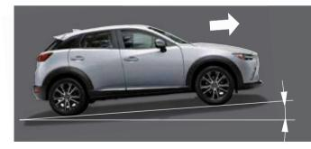
**IMPORTANT:** The HLA system will hold the vehicle for a maximum of two seconds while the driver is changing from the brake pedal to the accelerator pedal.
