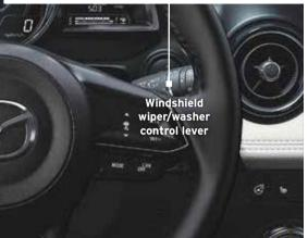
**NOTE:** Vehicles not equipped with AUTO wipers will have INT wipers. Set the lever to INT and choose an interval timing by rotating the ring between fast and slow.
