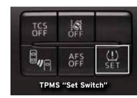
WHAT TO DO? Don't ignore the TPMS warning light. Stop and check your tire pressure (when tires are cold) and inflate the tires to the proper pressure. Properly inflated tires are safer, last longer, and increase fuel economy.
