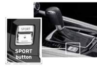
**NOTE:** If the SET button of the cruise control is pushed while in SPORT mode, SPORT mode is switched off. SPORT mode cannot be turned on or off when cornering.
