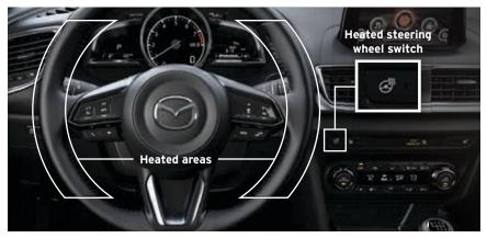
To turn heated steering wheel on: Push the switch and the light will illuminate. To turn heated steering wheel off:
