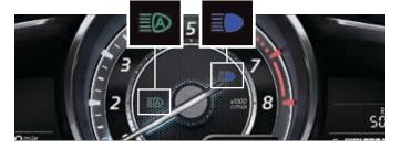
**NOTE:** When the HBC system is on, the HBC indicator light in the instrument cluster will illuminate (GREEN). The High Beam indicator light will turn on (BLUE) when the HBC system switches to high beam and will turn off when the HBC system switches to low beam.
