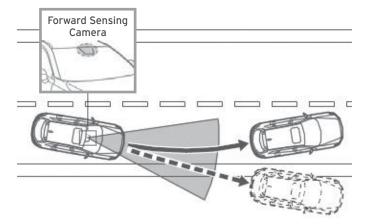
If the vehicle deviates from its lane at speeds above 37 mph, the system alerts the driver to provide steering assistance and uses the following indications to help the driver stay within the lines.
