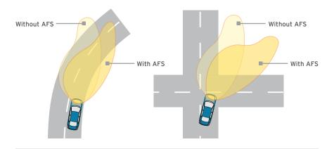
**NOTE:** With AFS, it is normal to see the headlights move and hear the sound of the headlight leveling motors at the front of the vehicle when the ignition is ON.
