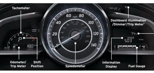
**IMPORTANT:** When your MAZDA CONNECT display setting is set on "AUTO", the instrument cluster and display may become dimmer when the headlights are on. If the display and instrument cluster become too dim or too bright when the headlights are on, simply rotate the dimmer knob located on your instrument cluster to adjust the brightness.
