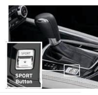
**NOTE:** If the SET button of the cruise control is pushed while in SPORT mode, SPORT mode is switched off. SPORT mode cannot be turned on or off when cornering.
