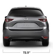
WHEELBASE (IN) 106.2 TRACK, FRONT (IN) 62.8 TRACK, REAR (IN) 62.8 LENGTH (IN) 179.1 WIDTH (IN) WITHOUT OUTER MIRROR 72.5 WIDTH (IN) MIRROR TO MIRROR OPENED 83.3 HEIGHT (IN) UP TO ROOF, WITHOUT ROOF RAILS 65.3 HEIGHT (IN) UP TO ROOF, WITHOUT ROOF RAILS, 66.1 UP TO SHARKFIN ANTENNA MINIMUM GROUND CLEARANCE - UNLADEN (IN) 7.5
