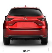
WHEELBASE (IN) 106.2 TRACK, FRONT (IN) 62.8 TRACK, REAR (IN) 62.8 LENGTH (IN) 179.1 WIDTH (IN) WITHOUT OUTER MIRROR 72.5 WIDTH (IN) MIRROR TO MIRROR OPENED 83.3 HEIGHT (IN) UP TO ROOF, WITHOUT ROOF RAILS 65.3 HEIGHT (IN) UP TO ROOF, WITHOUT ROOF RAILS, 66.1 UP TO SHARKFIN ANTENNA
