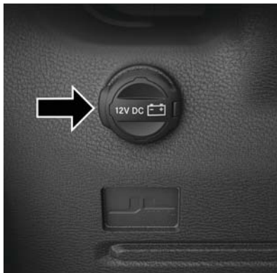
Rear Cargo Power Outlet
