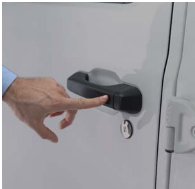
Push The Door Handle Button To Lock
