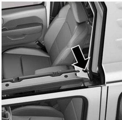
Torx Head Screw Location — Driver's Side Shown
