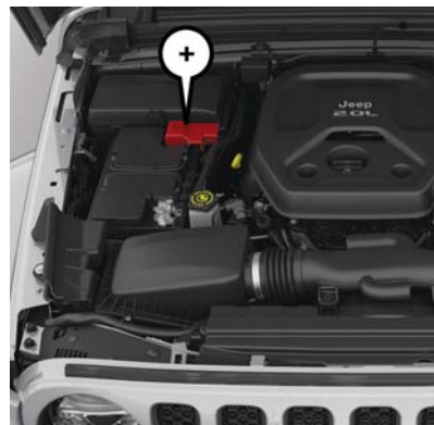
Positive Battery Post
