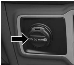
Front Power Outlet
