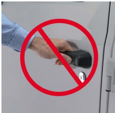
DO NOT Grab The Door Handle When Locking
