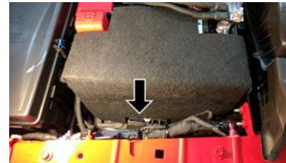
Auxiliary Switch Connections – Under Hood
