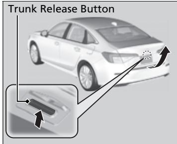
Push up the release button on the trunk lid after the doors are unlocked.
