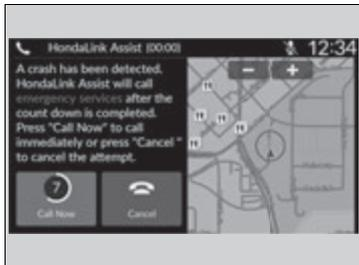
If your vehicle's airbags deploy or if the unit detects that the vehicle is severely impacted, your vehicle automatically will attempt to connect to the HondaLink operator. If connected, information about your vehicle, its location, and its condition can be sent to the operator\*1; you also can speak to the operator when connected.
