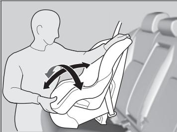
**6.** Make sure the child seat is firmly secured by rocking it forward and back and side to side; less than one inch of movement should occur near the seat belt.
