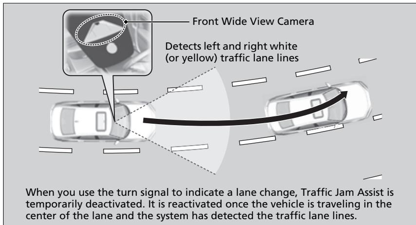
When the driver takes full control of the steering, the steering assist function is temporarily canceled.
