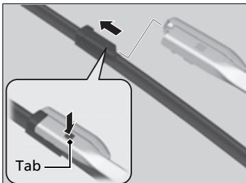
4. Depress the lock tab, then slide the wiper blade off the wiper arm.
