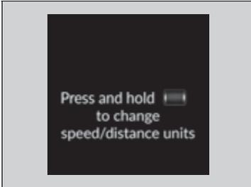
Enables you to show another unit on the driver information interface and set the displayed measurements to read in either miles and km, mph and km/h.
