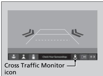
The system can be turned on and off on the audio/information screen by pressing the Cross Traffic Monitor icon.
