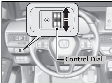
The brightness of the gauge is automatically adjusted depending on the ambient brightness.
