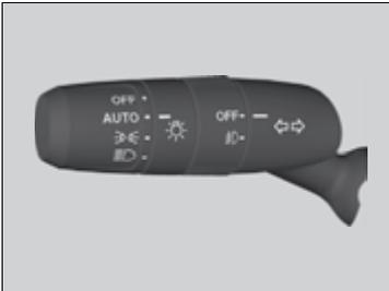
Automatic lighting control can be used when the power mode is in ON.
