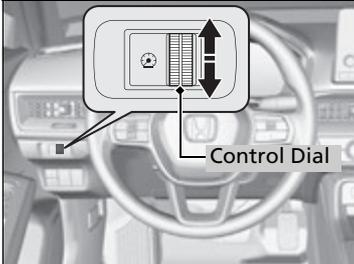
When the power mode is in ON, you can use the brightness control dial to adjust instrument panel brightness.
