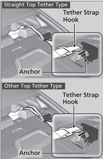
4. Open the tether anchor cover behind the head restraint.
