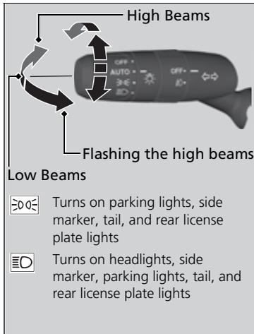
Rotating the light switch turns the lights on and off, regardless of the power mode setting.
