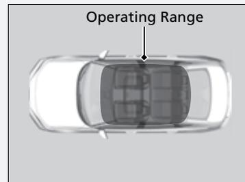
The engine may also start if the remote key is close to the door or window, even if it is outside the vehicle.
