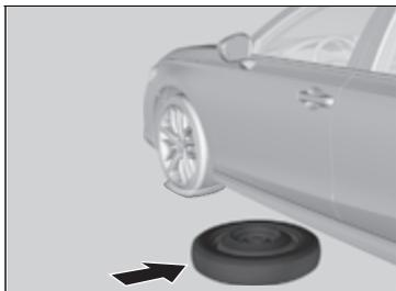
6. Place the compact spare tire (wheel side up) under the vehicle body, near the tire that needs to be replaced.
