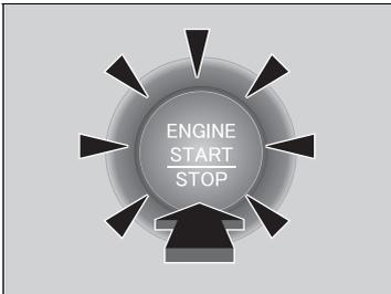
2. Depress the brake pedal and press the **ENGINE START/STOP** button within 10 seconds after the beeper sounds and the **ENGINE START/STOP** button changes from flashing to on.
