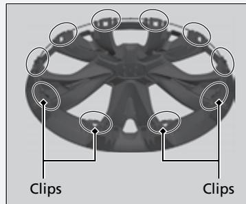
Align the valve mark on the wheel cover to the tire valve on the wheel, then install the wheel cover.
