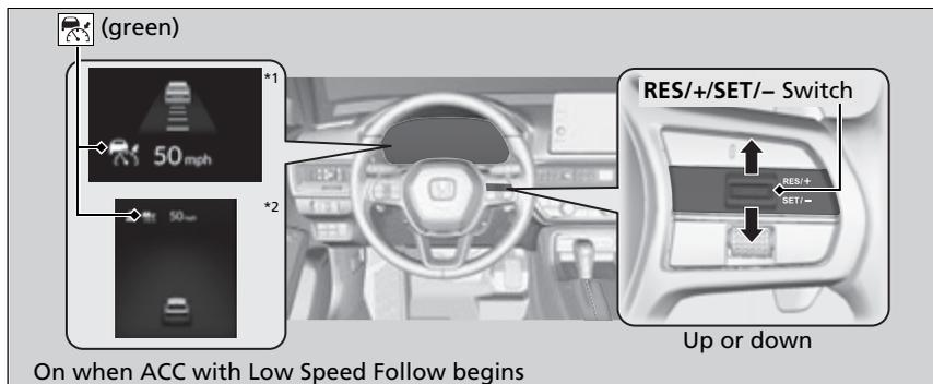
**When driving at about 25 mph (40 km/h) or above:** Take your foot off the pedal and press the **RES/+ / SET/-** switch up or down when you reach the desired speed. The moment you release the switch, the set speed is fixed, and ACC with Low Speed Follow begins.
