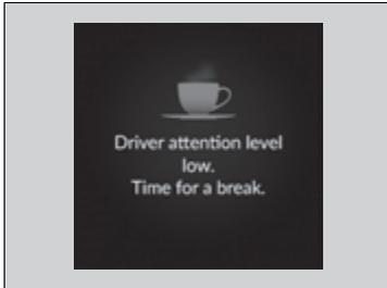
If one bar lights up, the **Driver attention level low. Time for a break.** message will appear, a beep will sound, and the steering wheel will vibrate.
