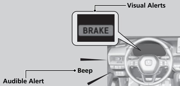
You can change the distance (**Long/Normal/Short**) between vehicles at which the system's earliest collision alert will come on through the driver information interface\* or audio/information screen\* setting options.
