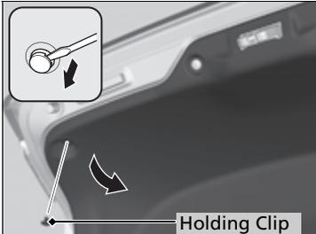
1. Remove the holding clip using a flat-tip screwdriver, then pull the lining back.
