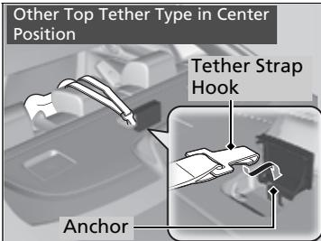
3. Secure the tether strap hook to the anchor.
