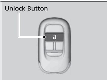
**To open:** Press the unlock button, and then within 10 seconds, press it again and hold it. If the windows stop midway, repeat the procedure.
