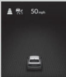
Your vehicle maintains the set speed without having to keep your foot on the brake or accelerator pedal.
