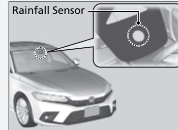
**AUTO** should always be turned OFF before the following situations in order to prevent severe damage to the wiper system:
