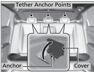
A tether anchor point is provided behind each rear seating position. If you have a child seat that comes with a tether but can be installed with a seat belt, the tether may be used for additional security.
