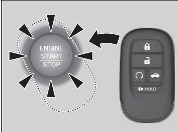
1. Touch the center of the **ENGINE START/STOP** button with the **H** logo on the remote key while the **ENGINE START/STOP** button is flashing. The buttons on the remote key should be facing you.
