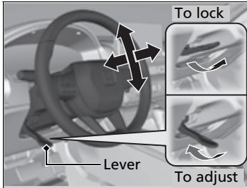
1. While the vehicle is stopped, push the steering wheel adjustment lever down.
