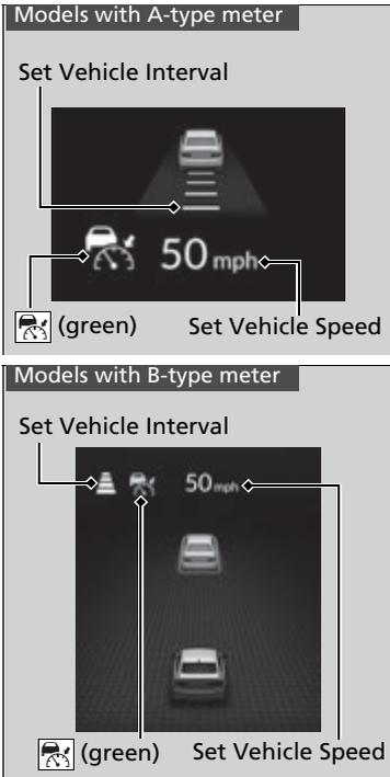
When ACC with Low Speed Follow starts operating, the vehicle icon, interval bars and set speed appear on the gauge.
