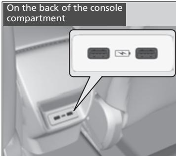
■ **On the back of the console compartment\***
