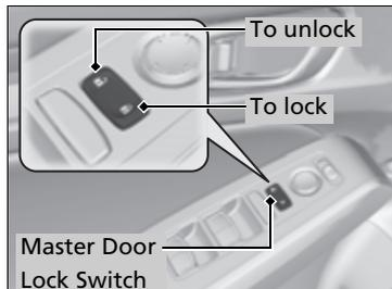
Press the master door lock switch in as shown to lock or unlock all doors and fuel fill door.
