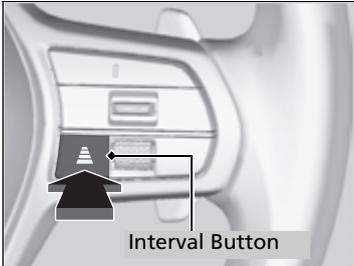
Press the Interval button to change the ACC with Low Speed Follow following-interval. Each time you press the button, the following-interval (the interval behind a vehicle detected ahead of you) setting cycles through furthest, far, mid, and nearest following-intervals.
