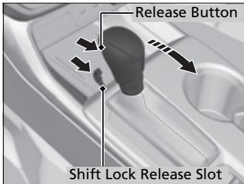
4. Insert the key into the shift lock release slot.
