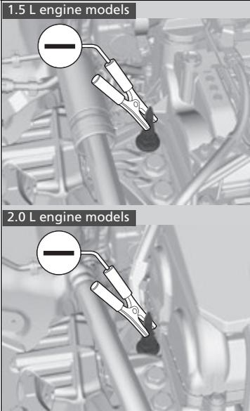
5. Connect the other end of the second jumper cable to the stud bolt as shown. Do not connect this jumper cable to any other part.
