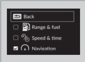
3. Roll the right selector wheel to scroll between contents, then press the right selector wheel to check or uncheck them.
