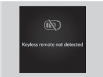
When the power mode is set to any mode other than OFF and you remove the remote key from the vehicle and shut the door, an alarm will sound. If the alarm continues to sound, place the remote key in another location.
