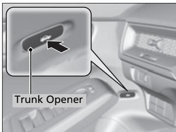
Press and hold the trunk opener on the driver's door to unlock and open the trunk.
