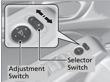
You can adjust the door mirrors when the power mode is in ON.
