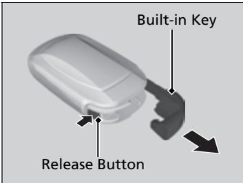
The built-in key can be used to unlock the doors when the remote key battery becomes weak and the power door unlock operation is disabled.
