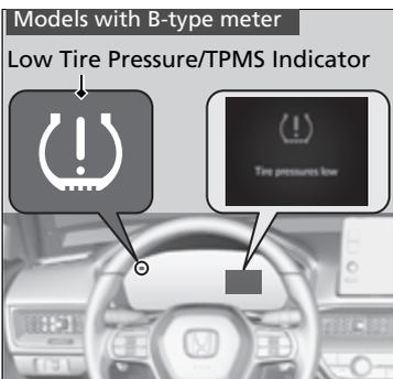
This will cause the low tire pressure/TPMS indicator to come on and a message to appear on the gauge.
