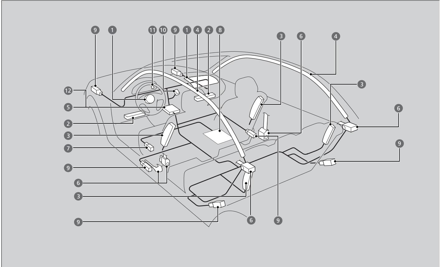
The front, front knee, side, and side curtain airbags are deployed according to the direction and severity of impact. Both side curtain airbags are deployed in a rollover. The airbag system includes:
