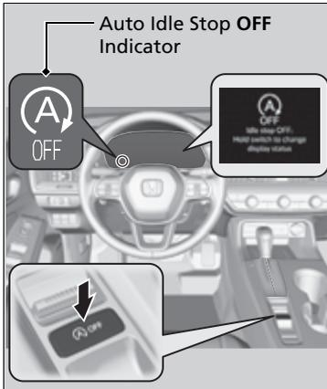
To turn the Auto Idle Stop system off, press this button. The Auto Idle Stop system stops.
