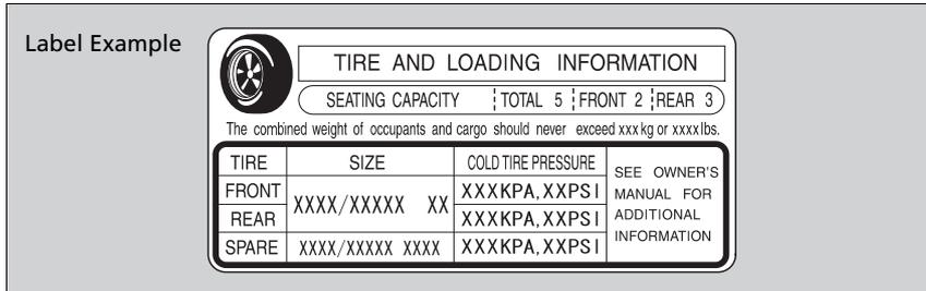
This figure includes the total weight of all occupants, cargo, and accessories, and the tongue load if you are towing a trailer.
