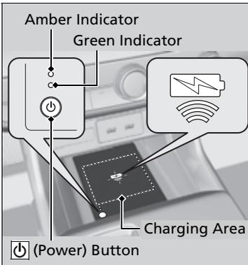
1. To turn the system on and off, press and hold the
