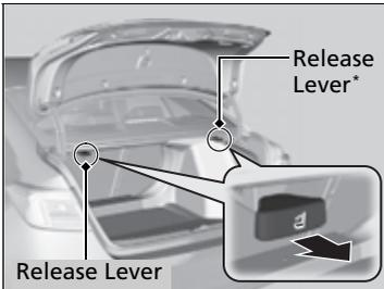
1. Pull the release lever in the trunk to release the lock.
