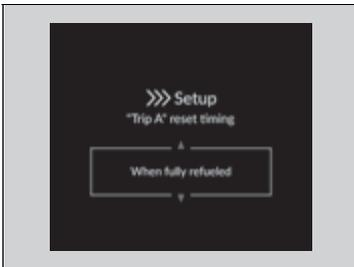
5. Roll the left selector wheel and select **When fully refueled**, then press the left selector wheel.
