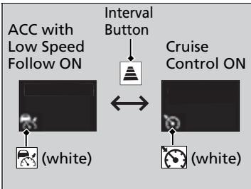
Press and hold the Interval button for one second. **Cruise mode selected** appears on the driver information interface for two seconds, and then the mode switches to Cruise.
