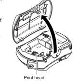
Insert four new AAA-size alkaline batteries (LR03), making sure that their poles point in the correct directions. Always replace all four batteries at the same time using brand
