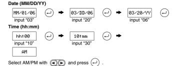
You can also confirm the figure and move to the next setting by using right cursor key.
