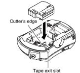
Make sure that the end of the tape feeds under the tape guides · Use only Brother M tapes with this machine. Attach the back cover by inserting two
